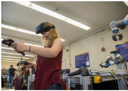
Figure 1: In addition to providing alternative interfaces for remote teleoperation and offline programming, technologies such as virtual reality provide feedback mechanisms useful for teach-by-demonstration interactions.
